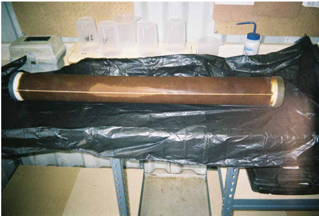
Figure 4-21. Spent Media Cartridge Removed from Isolux™ System (Provided by MEI)
