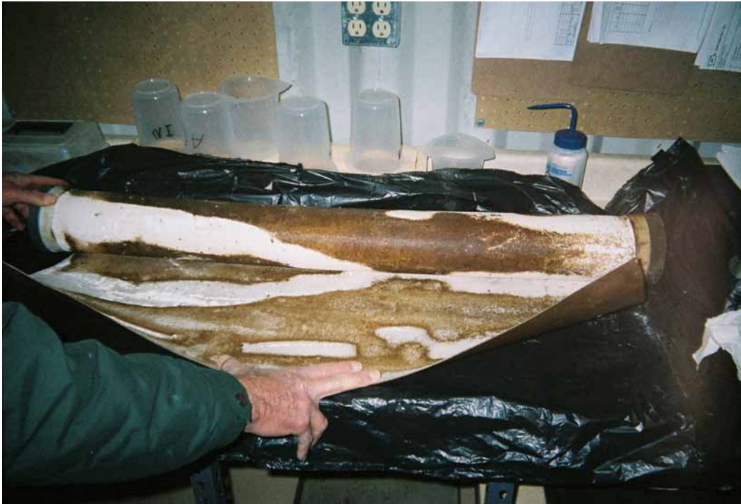
Figure 4-22. Spent Media Cartridge with Outer Membrane Cut Away (Provided by MEI)
